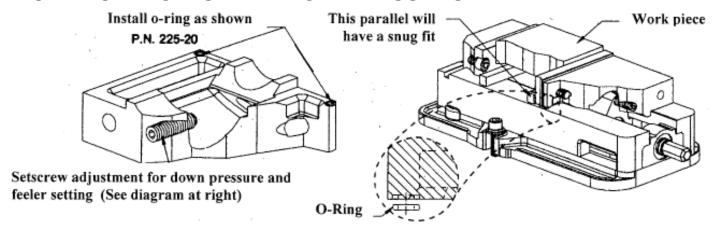
Most jobs require a tight contact between the workpiece and the parallels (see above). This option offered by Kurt Manufacturing Company is ideal for that. The O-Ring installation will provide for the movement needed when working with parallels.
