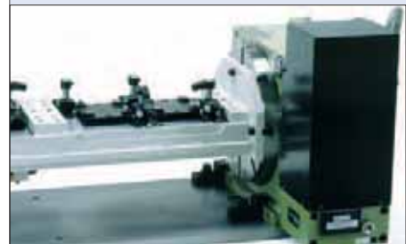
Solution: Up to three-sided machining using an indexing trunnion fixture.
