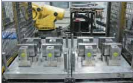
Solution: Second operation grinding fixture feeds productivity into FMS.
