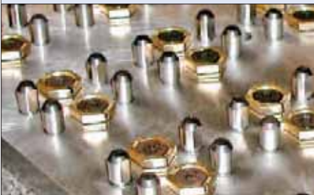
Solution: High density fixture clamping four parts per station.
