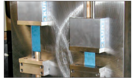
Solution: D100 movable and stationary jaws integrated onto a tower.
