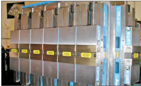
Solution: High density DoubleLock vise setup holds 18 parts for precision machining.
