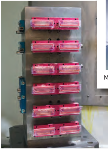
DoveLock jaws used for glass machining
