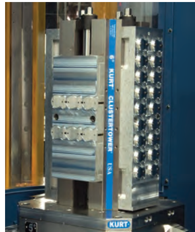
Cluster Tower using fixture plate & Soft jaws
