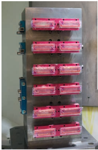
DoveLock jaws used for glass machining
