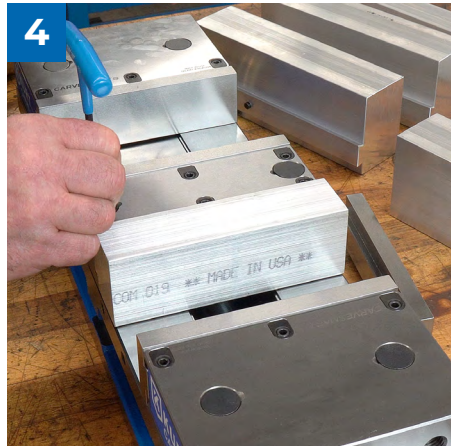
4 Then firmly tighten all screws. Do the same with each individual jaw plate and you're ready to go.
